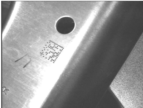
Individual Part Marked with Data Matrix
